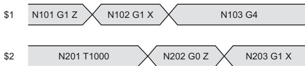
Timing diagram in manual arbitrary reverse run
